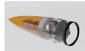
Figure 4. Redesign of nose cone to have a removable payload
